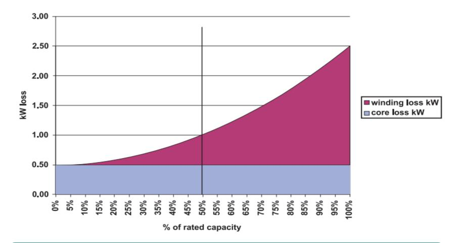
Both **No-Load and Load losses** of transformer are provided by manufacturer in test certificate.
