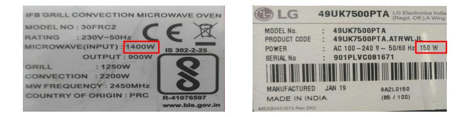
$$Input Power (kW) = \frac{Input Power (Watt)}{1000}$$
