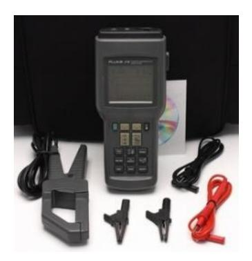
**Usage:** Can be used to measure instantaneous power of any kind of loads  $(1\emptyset \text{ or } 3\emptyset)$ . No provision for data recording.
