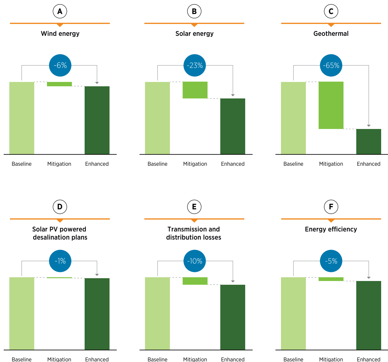
Figure 19: GHG reduction potential of individual mitigation option in 2030 compared with the baseline scenario (in %)
