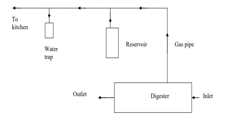
Approximately, one person will generate one kg of kitchen waste and 20 kg of kitchen waste will generate 1.2 lb of LPG equivalent of biogas daily
